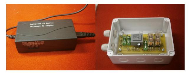
The solenoid valve and the optosensors are working on 24V DC voltge. We can offer a simple 24V notebook charger for this purpose or we can manufacture individually sutch device.
