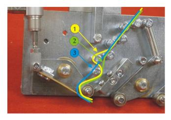
The green line (2) is the usual way. This solution can be used with the most tapes and sheets.
