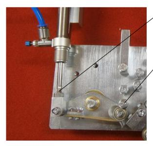
You can set the end position of the moving roller with turning around the axle of the pneumatic cylinder after loosing this nut.
