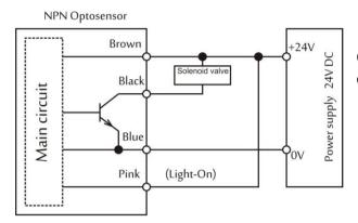
Connecting OMRON E3F1-TN series optosensor.
