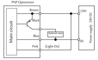
Connecting OMRON E3F1-TP series optosensor.
